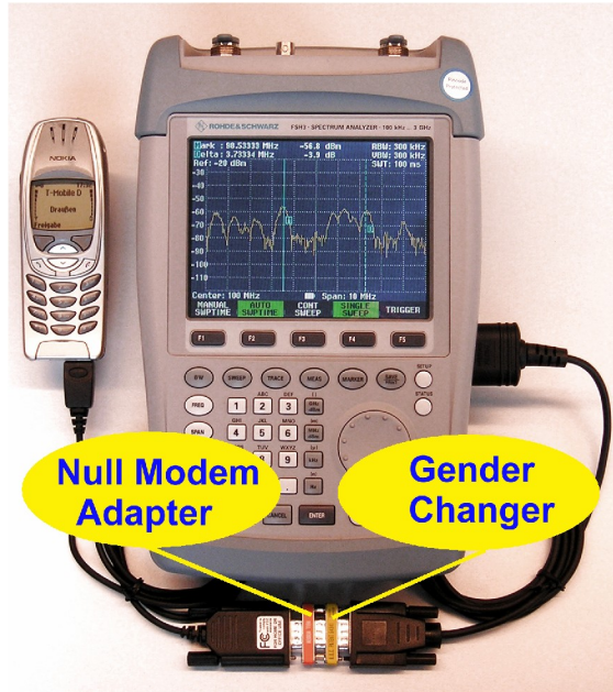
Fig 6 Connect the FSH to a modem or mobile phone using a null modem adapter (crosslink cable) and a male-male gender changer
